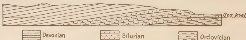
FIG. 427.—A Section in New York state showing the relation of the Ordovician, Silurian, and Devonian. (After W. J. Miller.)
